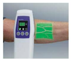
AN ACCUVEIN DEVICE reveals hard-to-find veins, enabling faster, more accurate needle placement.
